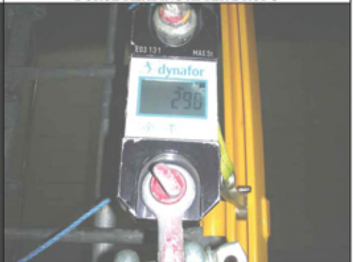
START OF DROP 6 -- HIGH READING DUE TO LIFT
